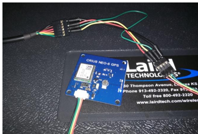
Figure 3: Connected Tx, Rx, Vcc, and Gnd lines
