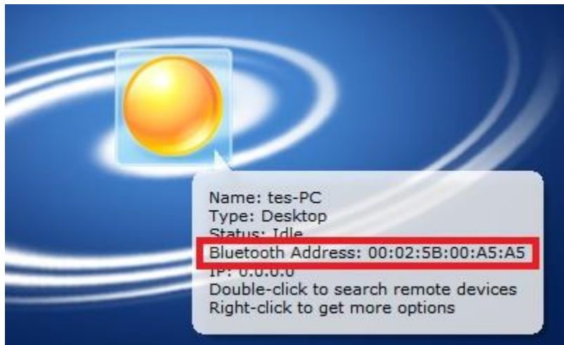
Figure 2: Default Bluetooth MAC address shown in BlueSoleil BT stack
