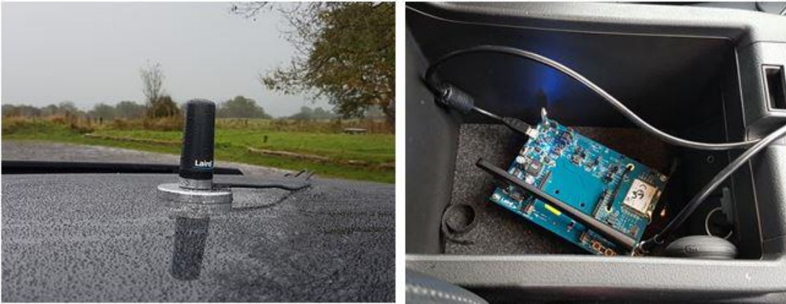
Figure 3: RM186 development board setup including antenna mounted on car roof
