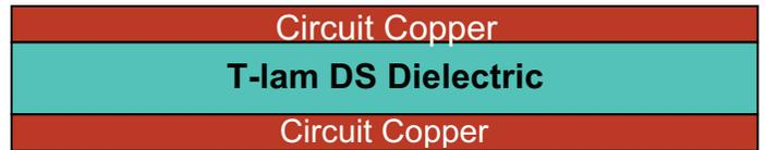
FIGURE 3: Tlam ML Circuit Illustration
